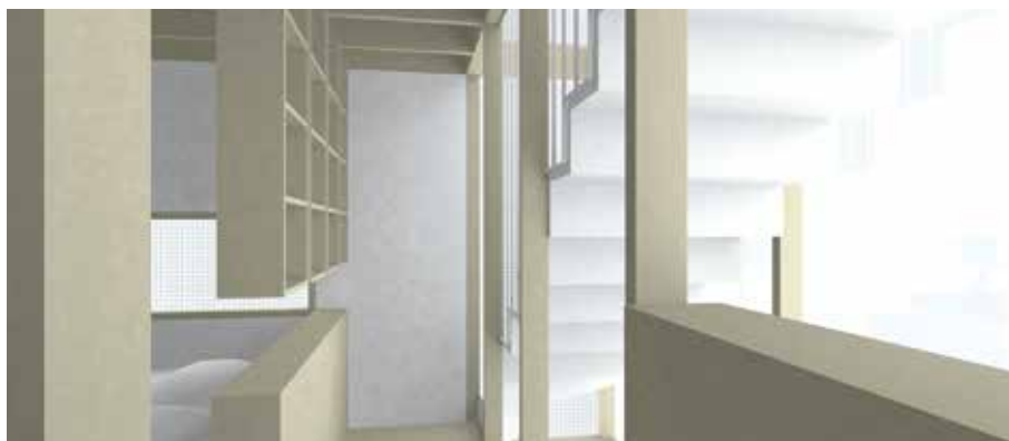
A dual-skin staircase acts as a climatic buffer from thermal gains, and allows diffuse light into the bedroom.
